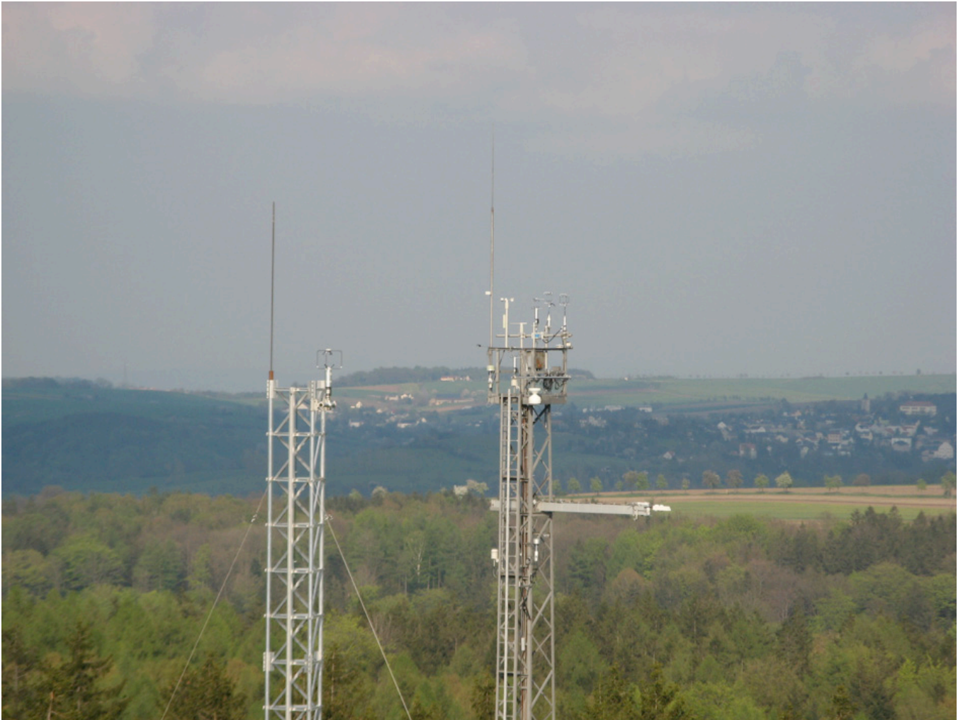
Measuring towers of the TU Dresden (Chair of Meteorology) in the Tharandter Forest to determine the water and carbon flows. Photo: Ronald Queck
